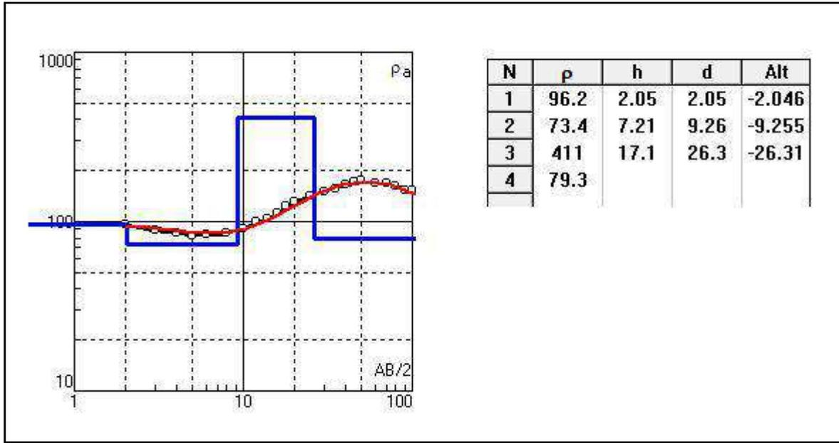
**Fig-6.5:VES Curve and interpreted results at Badadhara (Near Coal Yard, Outside of plant area)(VES3)**
