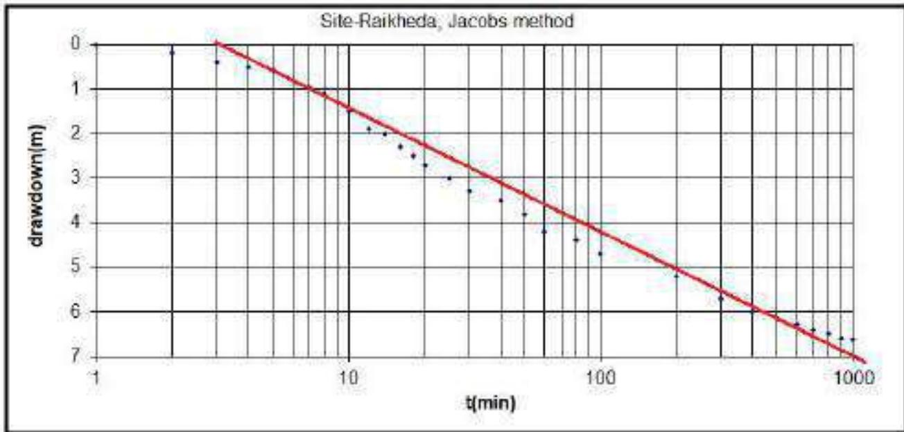
The pumping test data has been analyzed by Jacob's straight line method of the pumping data of the observation well. The calculation is given below.
